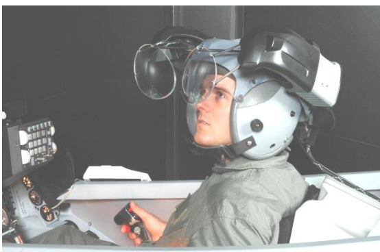
Figure 12 A Helmet-mounted Visual System
