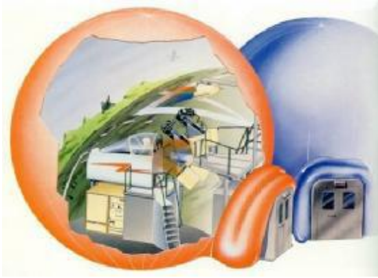
Figure 11 Military Dome Projection System
