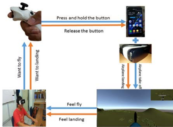
Fig 6. Architecture of Virtual Reality Flight Simulator
